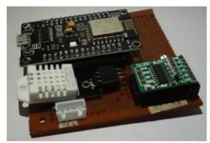
Figure 3. NodeMCU based hardware system.
