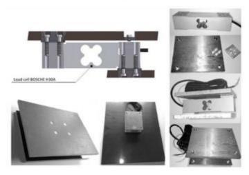
Fig. 1. Load cell assembling process
