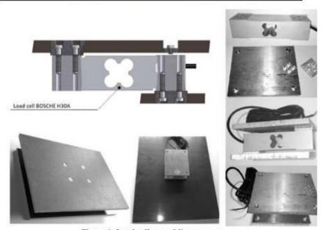
Figure 1. Load cell assembling process
